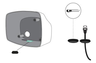
Make an incision in the rubber plug and insert the ethernet cable without the RJ45 connector. Make sure the cable is not too tight and has some clack to facilitate reopening the cover for possible maintenance or servicing. Crimp the RJ45 connector to the cable and connect the cable to the ethernet port in the charger.
