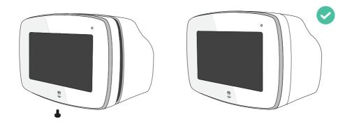
Recommended tightening torque 0.7 Nm +/- 10%
