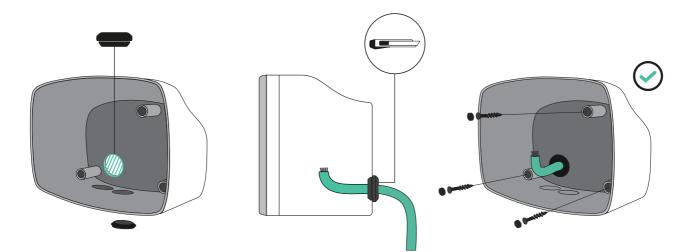
Fix the charger on the wall using the appropriate screws.
